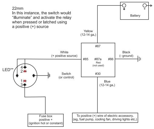
\*\*Note: The LED connections are NOT polarity sensitive on the 22mm switches (one is to be a positive connection and the other is to be a negative connection)
