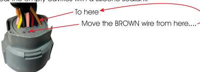
The round gray plug is now ready to connect to a 4L80E transmission. The 4L80E transmission has two speed sensors vs. one on the 4L60E. You will now have two "extra" wires. (TAN & WHITE) These will be used for the 4L80E's INPUT speed sensor.
