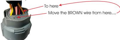
The round gray plug is now ready to connect to a 4L80E transmission. The 4L80E transmission has two speed sensors vs. one on the 4L60E. You will now have two "extra" wires. (TAN & WHITE) These will be used for the 4L80E's INPUT speed sensor.
