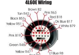
3) **MOVE** the BROWN wire to the location where the white wire was. (the one removed in step 2)
