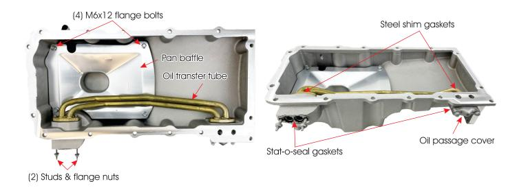
Install the oil pan gasket (not supplied) to the oil pan with a few bolts to hold in place. Apply a small bead of RTV sealant on the protruding front cover gasket (where the front cover meets the block). Do the same at the rear of the block (rear cover to block gasket).
