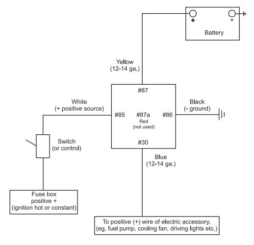
Note: Harness wire colors subject to change. Always compare with the terminal numbers (85,86,87,30) for reference. Terminals #85 and #86 can be "reversed" (eg. #86 + and #85 -) as long as one is positive and one is negative.
